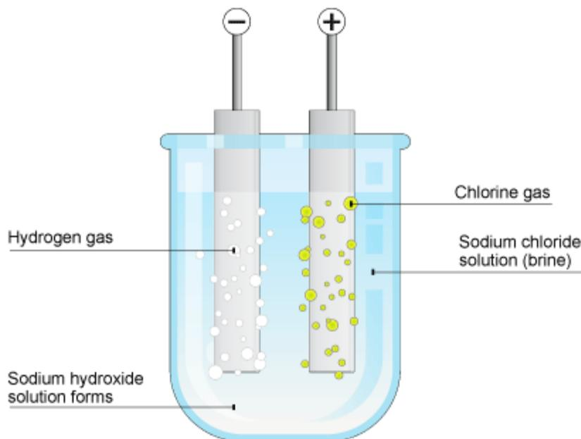
Electrolysis of sodium chloride solution
