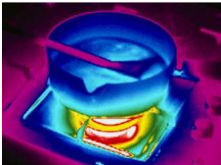
Thermogram of a pan being heated on a stove
