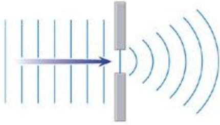
Diffraction through a narrow gap
